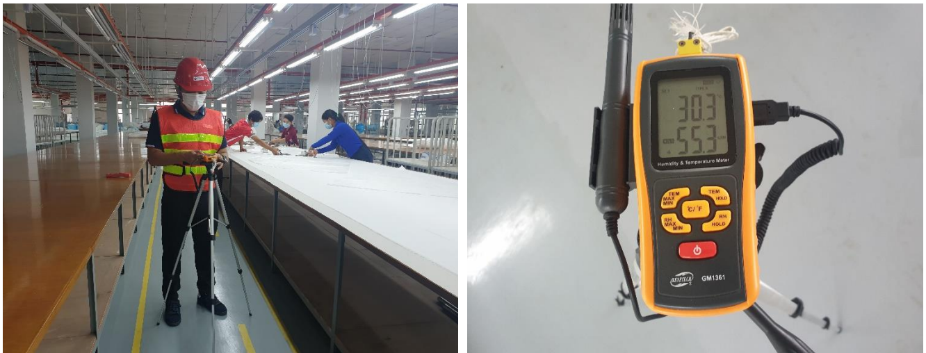
Figure 4-1 Temperature and Humidity Measurement in Operation Area of the factory
