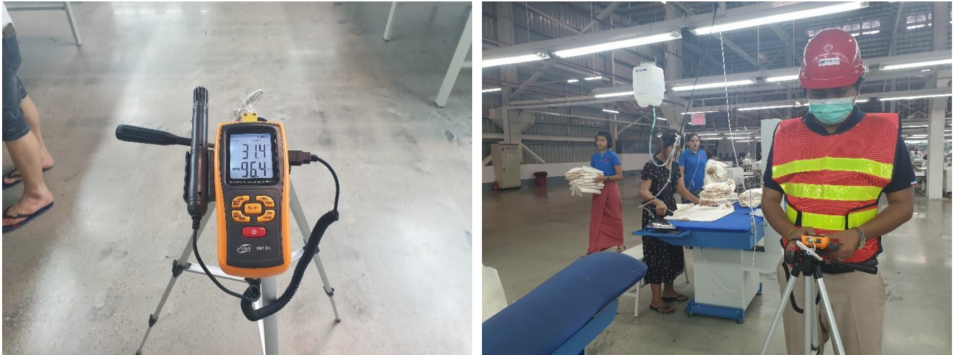
Figure 4-1 Temperature and Humidity Measurement in Operation Area
