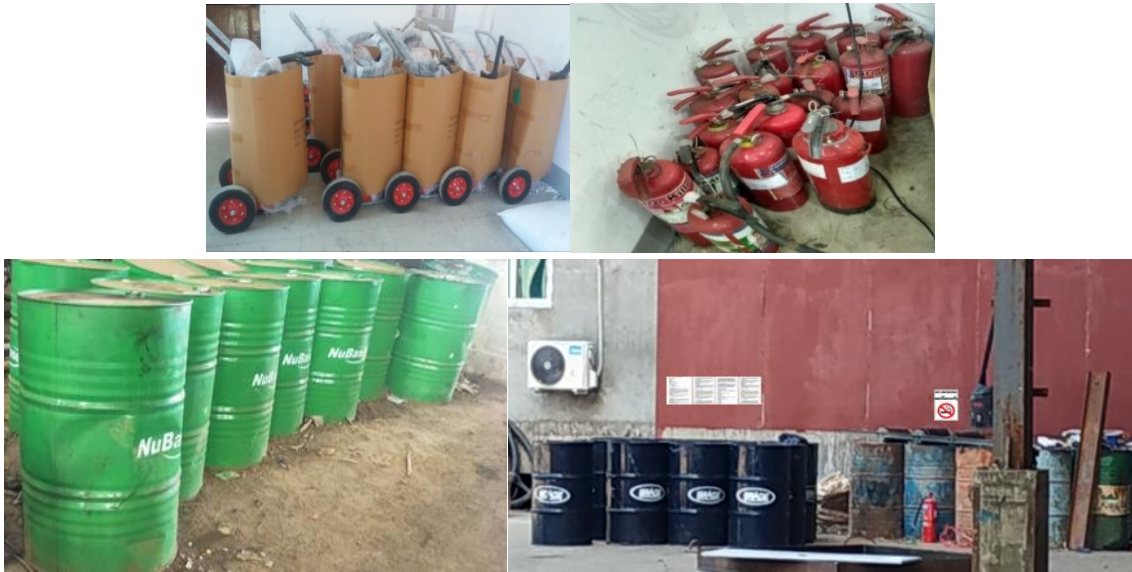
Figure 5.35 Lubricating Oil Storage Post with MSDS, Safety Signs and Extinguishers
