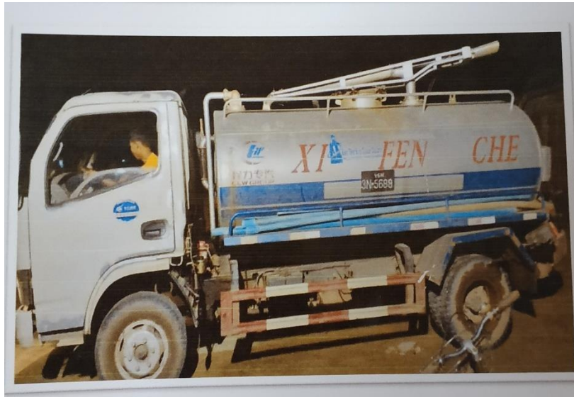
Figure 5.41 Photo Records for Sludge Waste Removal from Septic Tanks
