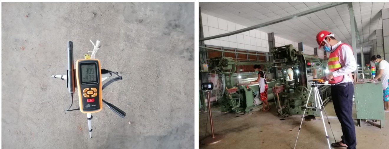
Figure 4-9 Temperature and Humidity Measurement in Operation Area of the Factory
