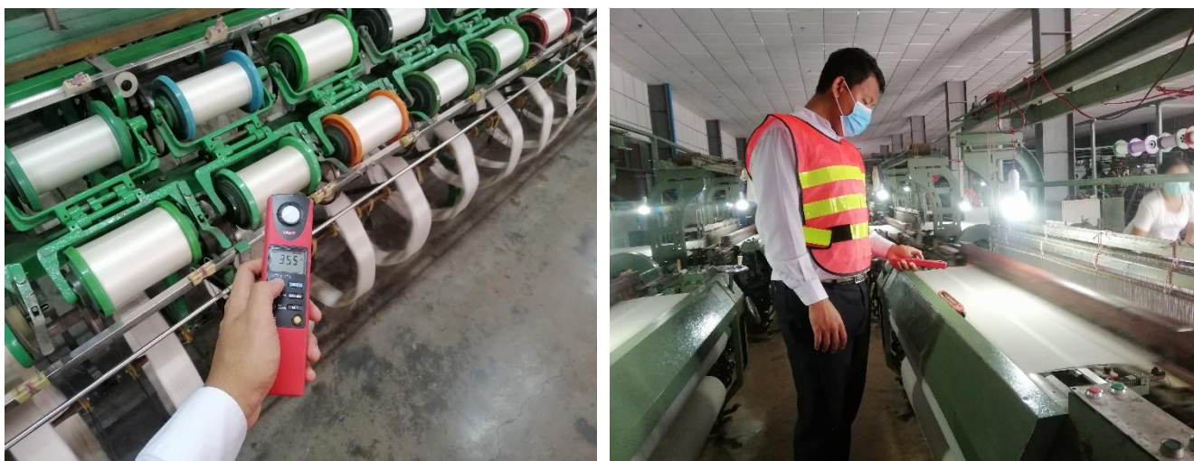
Figure 4-11 Light Quality Measurement of the factory
