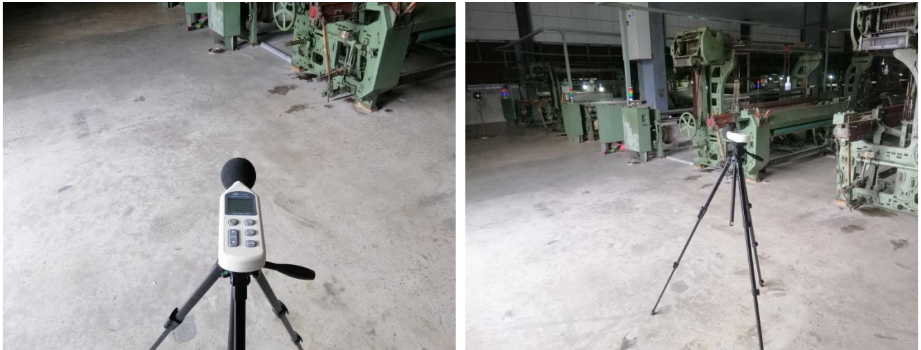
Figure 4-12 Noise level Measurement in the Factory
