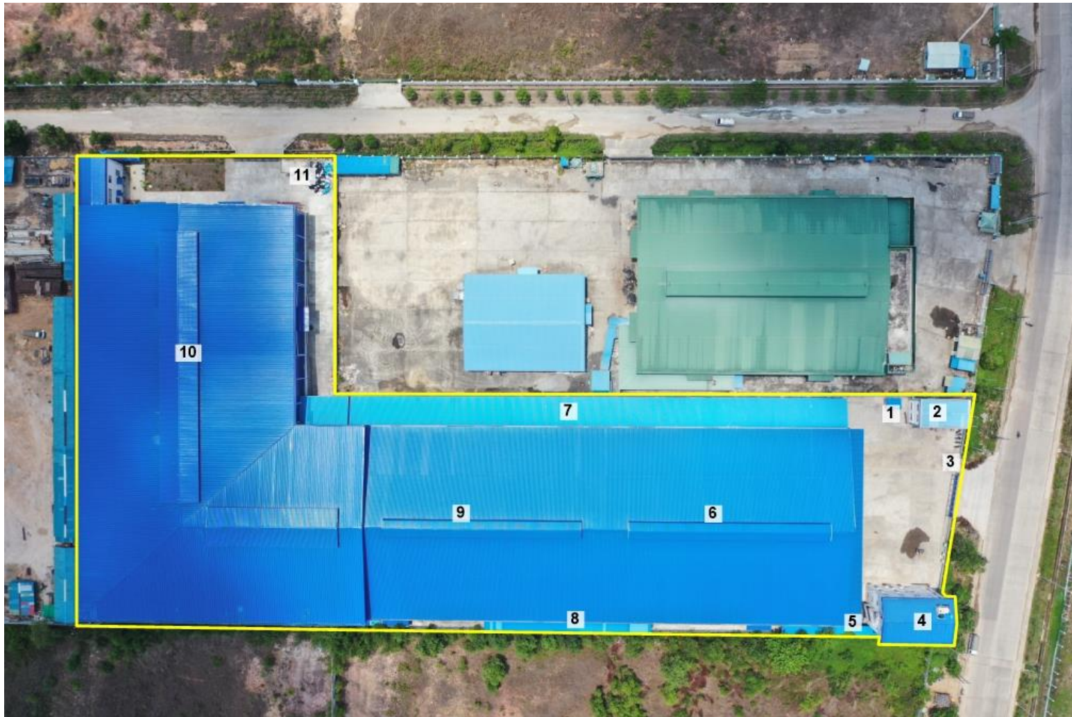
1.Underground Water Tank 2.Generator & Transformer Room 3. Security Gate 4.Dormitory 5.Fire Safety Pump 6.Products Warehouse 7.Canteen 8.Toilets 9.Office Room 10.Production Area 11.Solid Waste Storage Area
