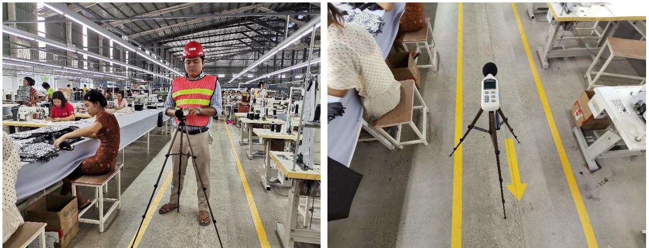
Figure 5-4 Sound level measurement photo
