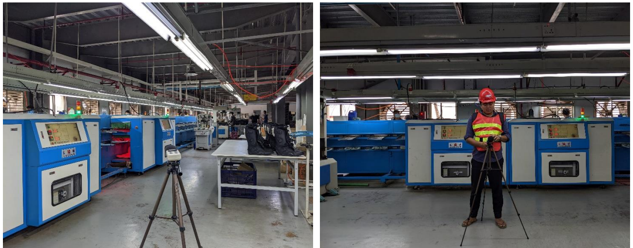
Figure 4-4 Sound level measurement photo
