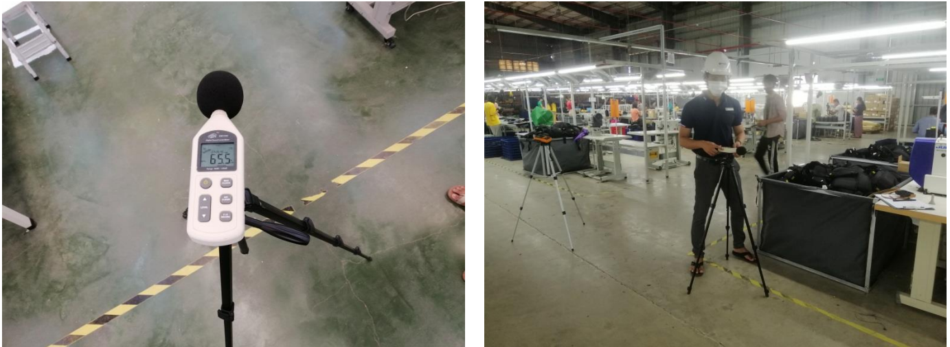
Figure 4-2 Indoor Noise Measurement of the project
