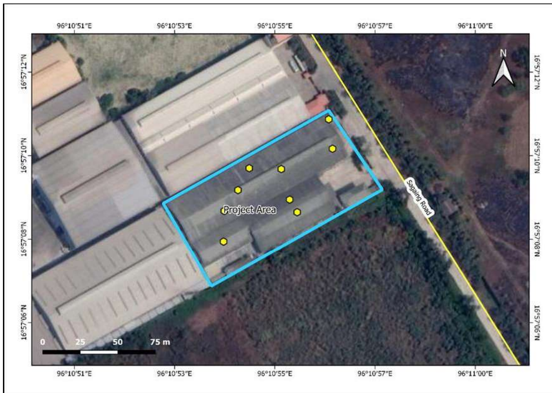
Figure 4-11 Noise quality measurement stations
