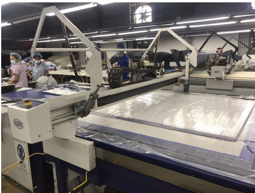
Figure 2-10 Cutting Used by Fully Automatic and Cutter Machine
