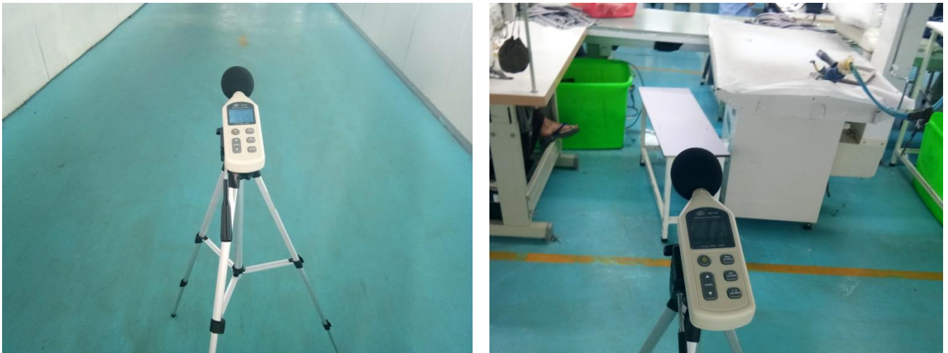
Figure 4-3 Sound Level Measurement Photo
