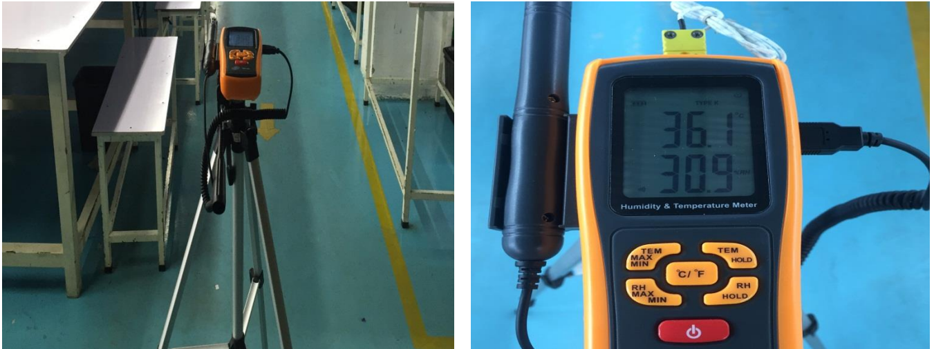
Figure 4-1 Temperature and Humidity Measurement in Operation Area
