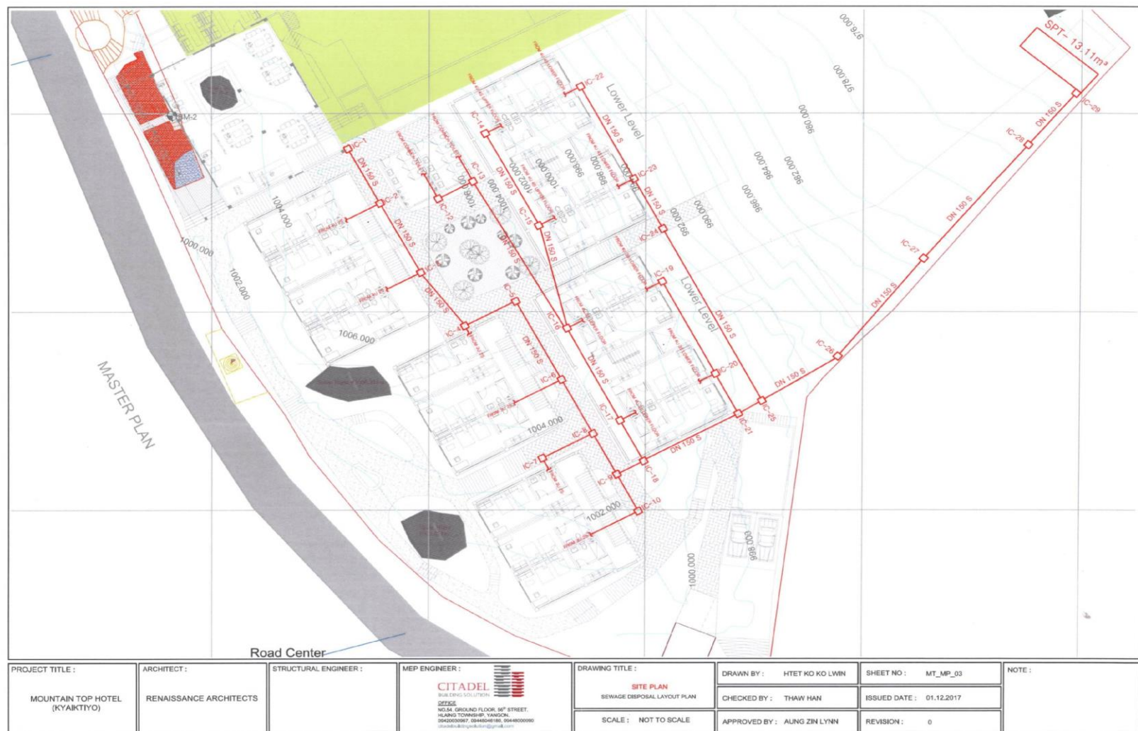
Fig.12 Sewage Disposal Layout Plan
