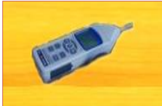
Figure 6.14 Photos of Noise Monitoring Device
