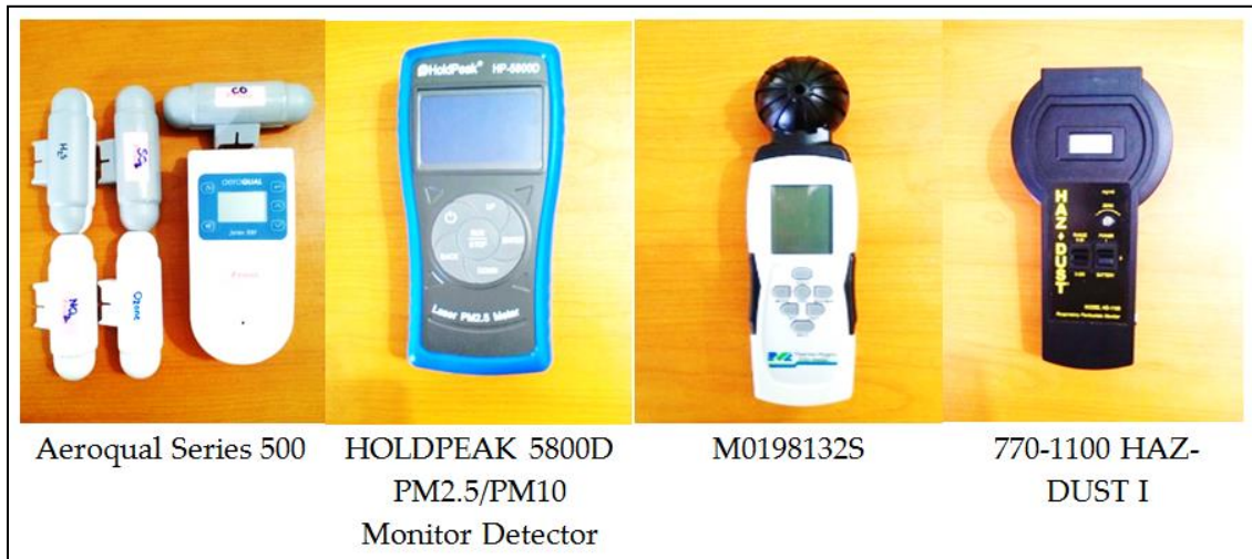
Figure 6.12 Photos of Air Monitoring Devices
