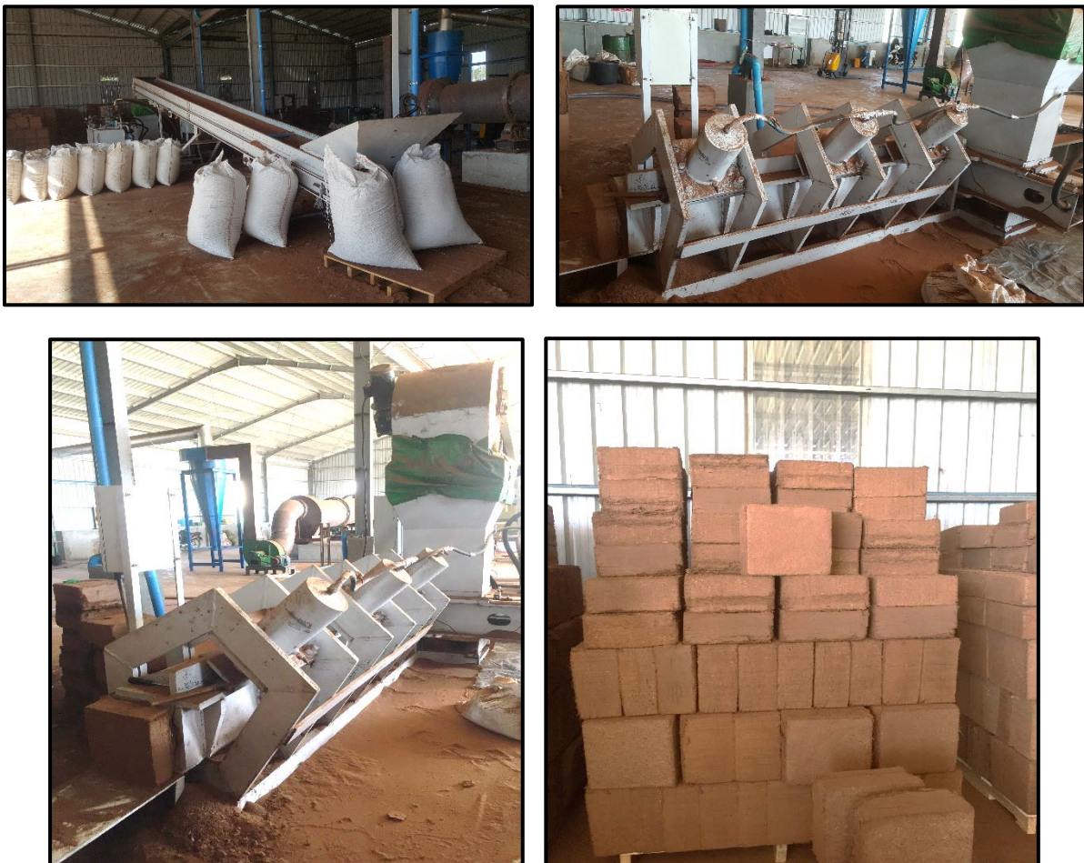
Figure 2-12 Conveyor Belt, Horizontal Compressor and Compacted Blocks
