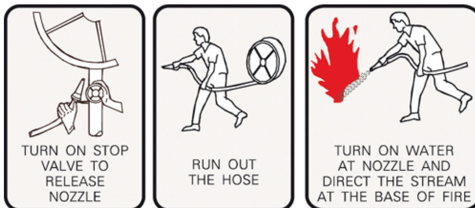
Figure 9-3 To Operate Fire Hose Reel
