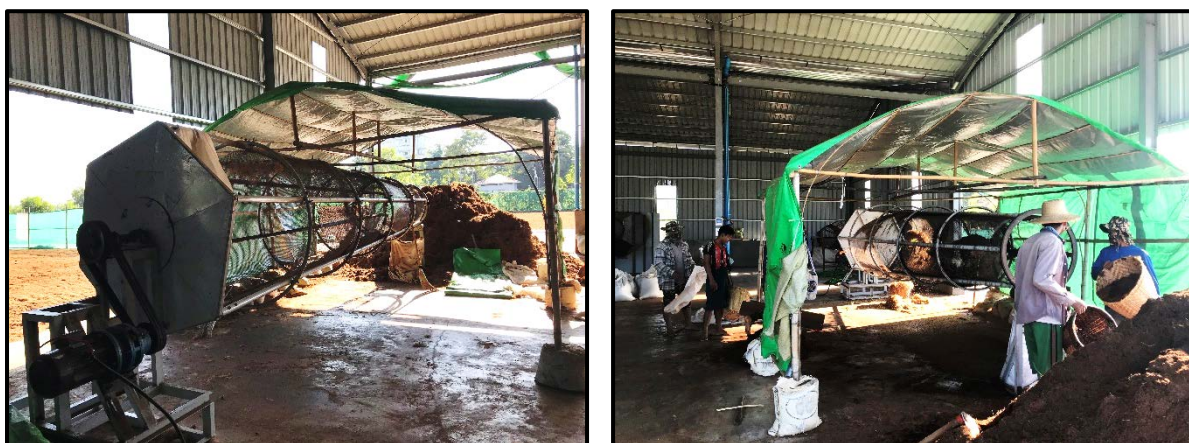
Figure 2-10 Screening with Rolling Filter
