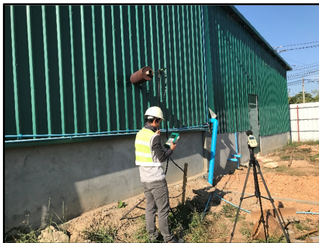
Figure 4-5 Generators Stack Emission Monitoring
