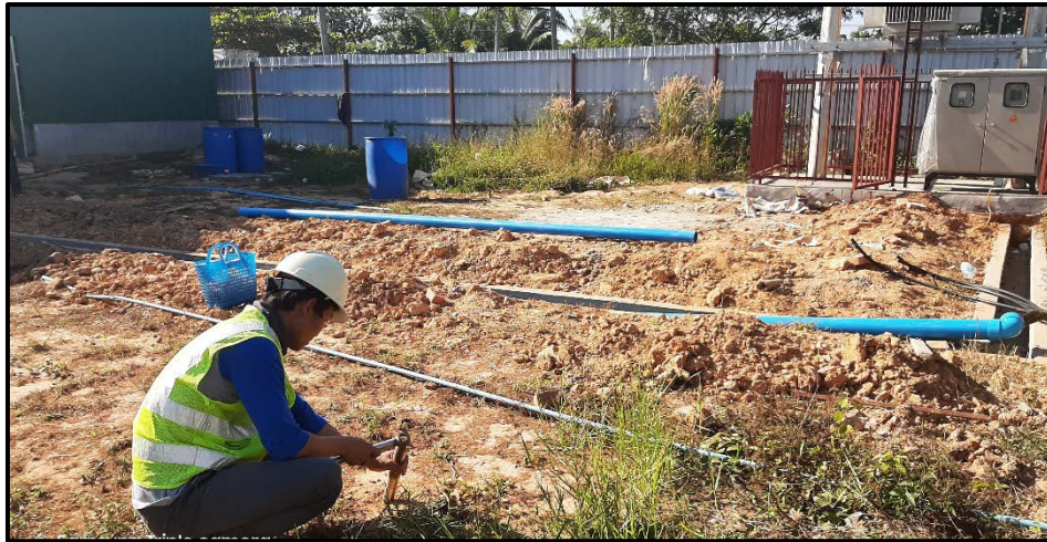
Figure 4-8 Photos of Taking Soil Sample inside of Factory Premise
