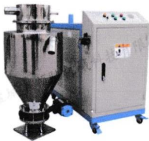
Raw Material Suction System and Feeding System
