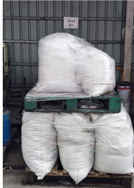
Figure 4.27: Storage of Boiler ash before collected by YCDC
