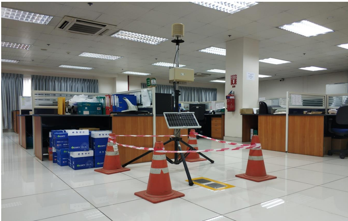
Figure 5.15: Ambient air monitoring at Office room
