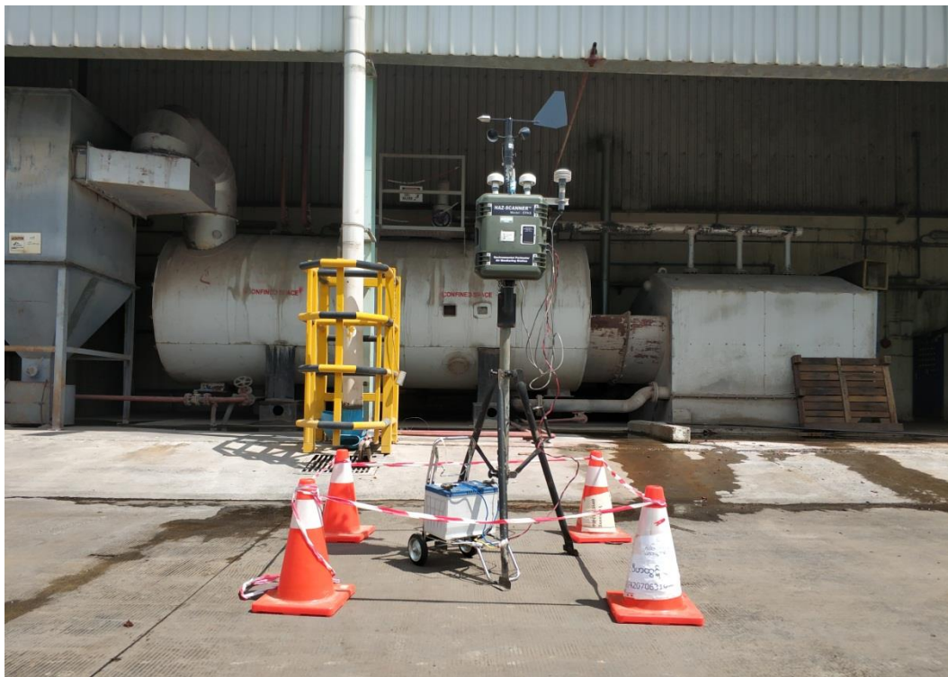
Figure 5.9: Ambient air monitoring near by the boiler
