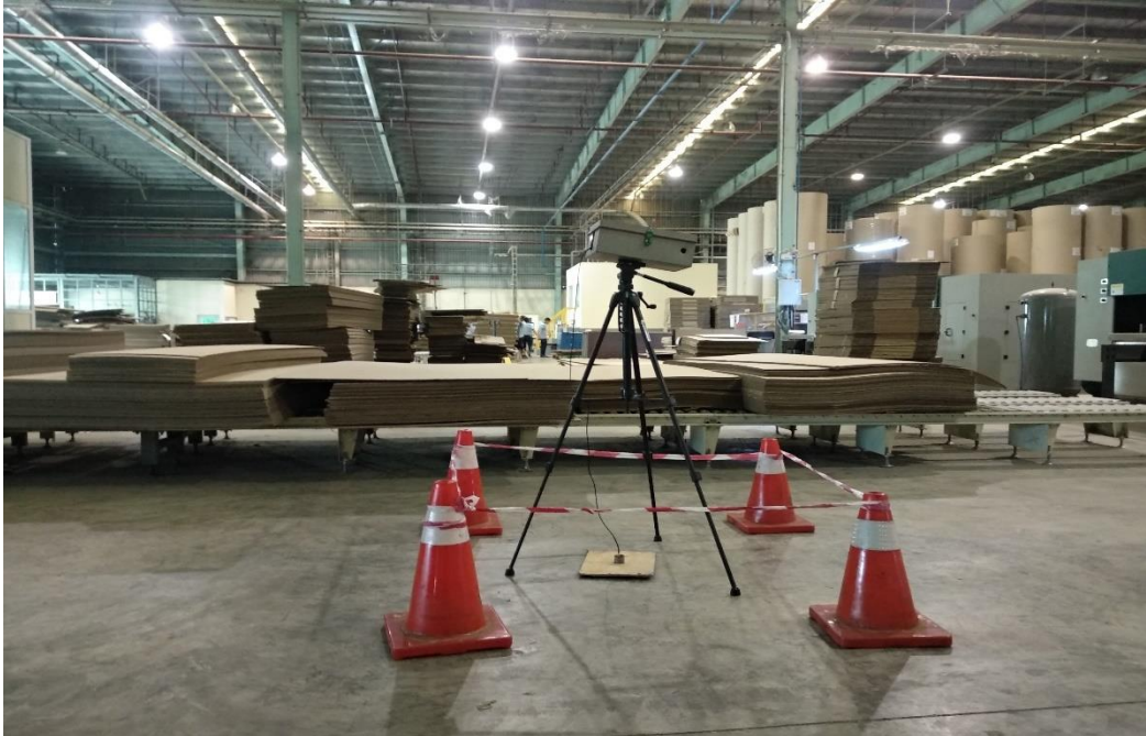
Figure 5.27: Vibration monitoring station at production area
