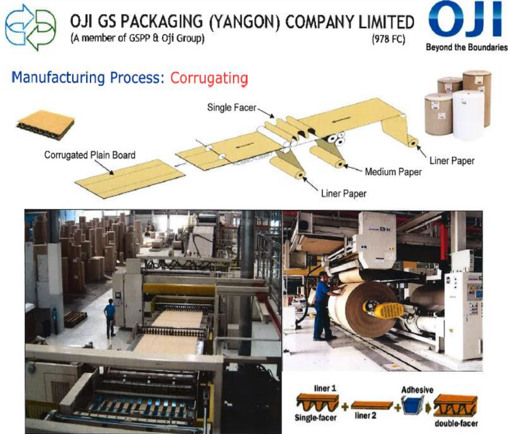
Figure 4.15: Corrugating step in operation phase
