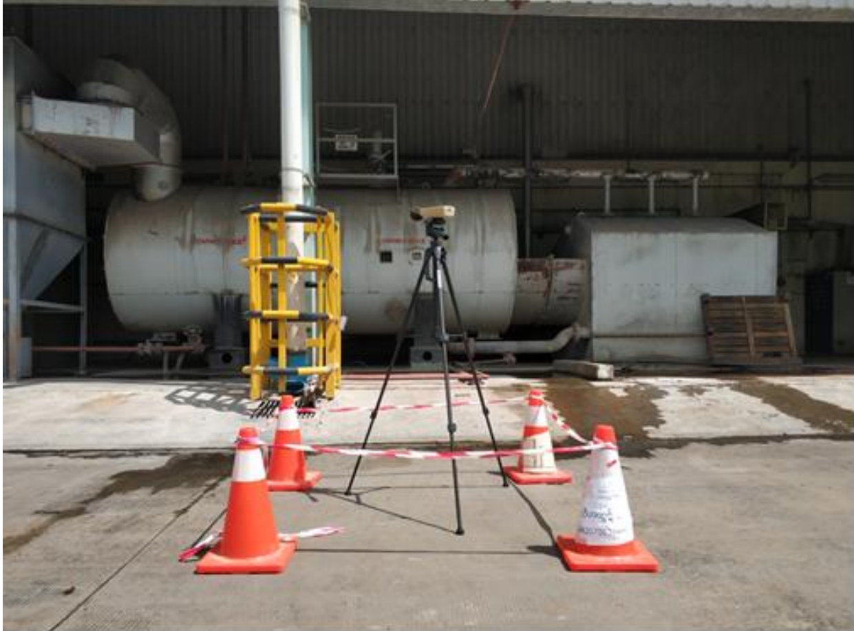
Figure 5.25: Noise monitoring station at factory boiler area
