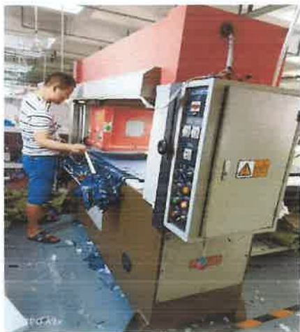
XCIP3 gantry-travelling type four column hydraulic press
