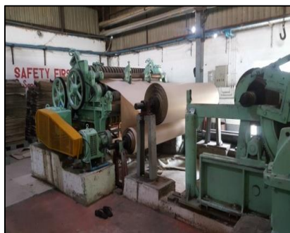
Figure 4-36: Reeling the Pulp on the Steel Axle
