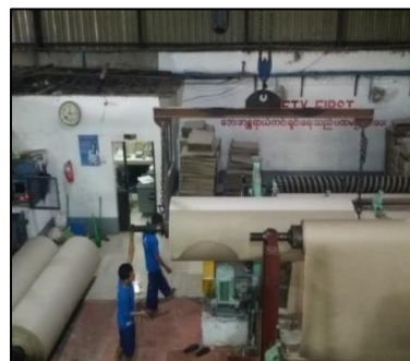
Figure 4-36: Reeling the Pulp on the Steel Axle
