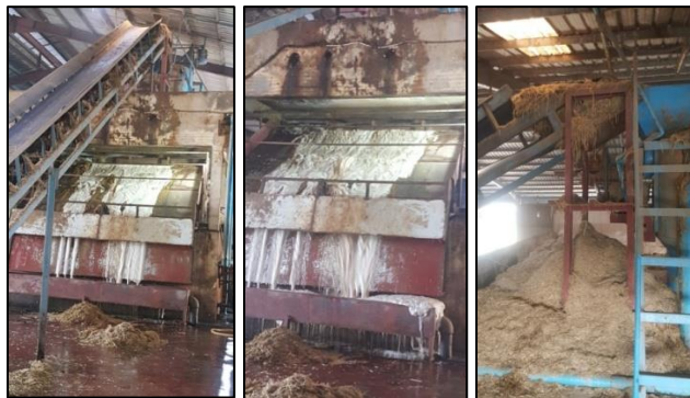
Figure 4-26: Washing the Chipped Straw with Diluted Black Liquor in the Straw Washer
