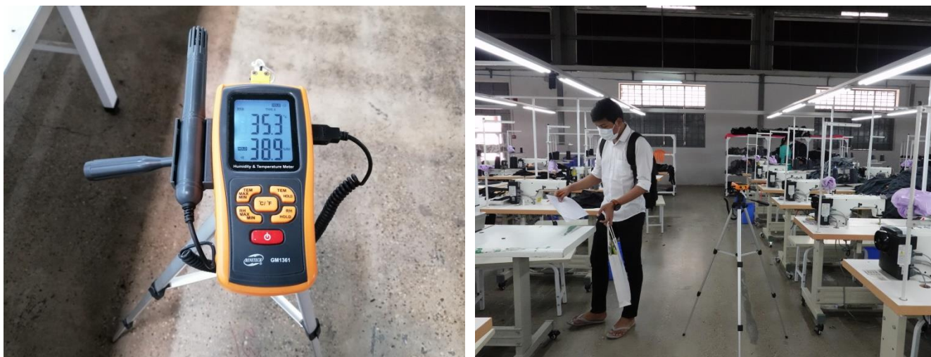
Figure 4-3 Temperature and Humidity Measurement
