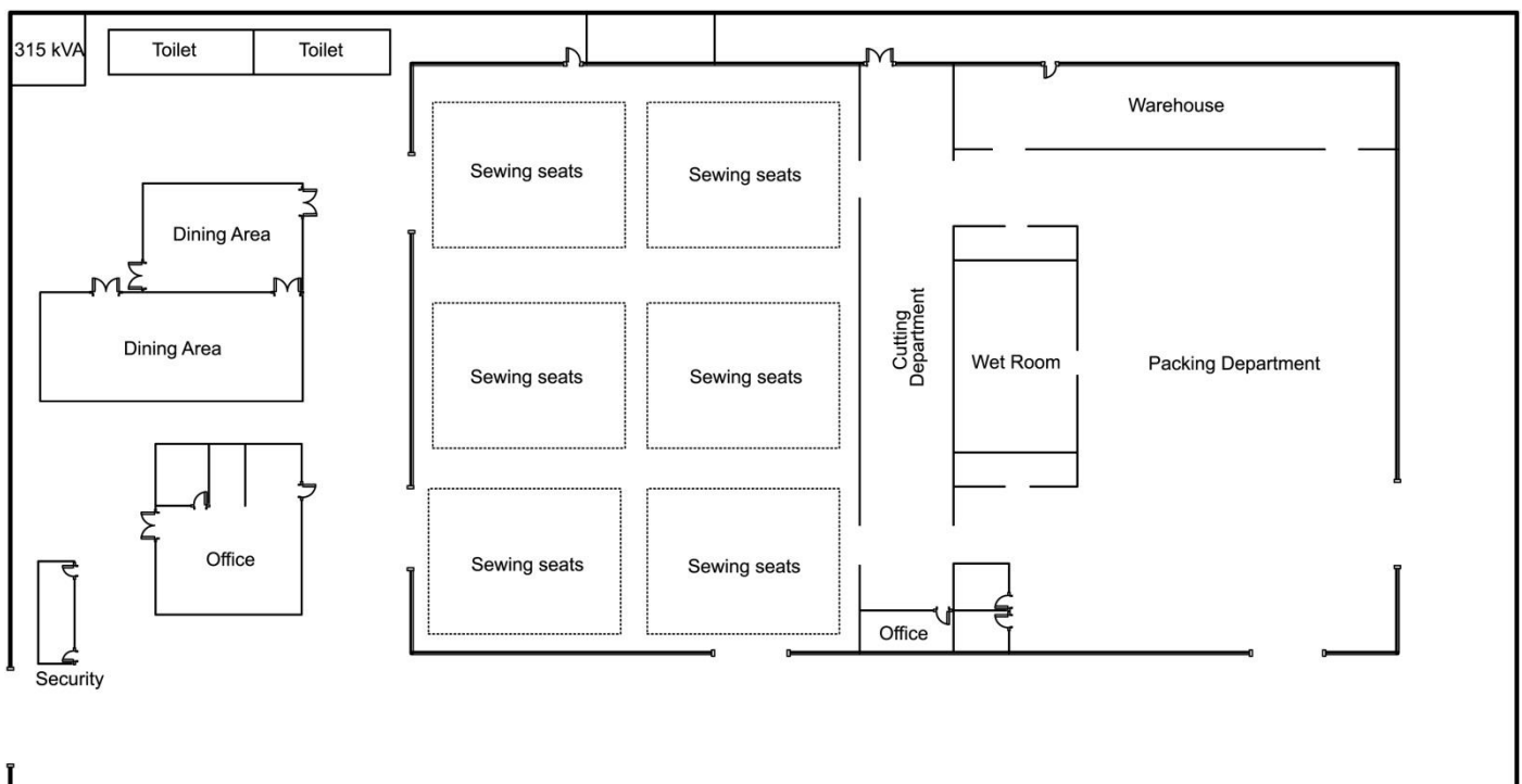
Figure 3-3 Factory Layout Drawing
