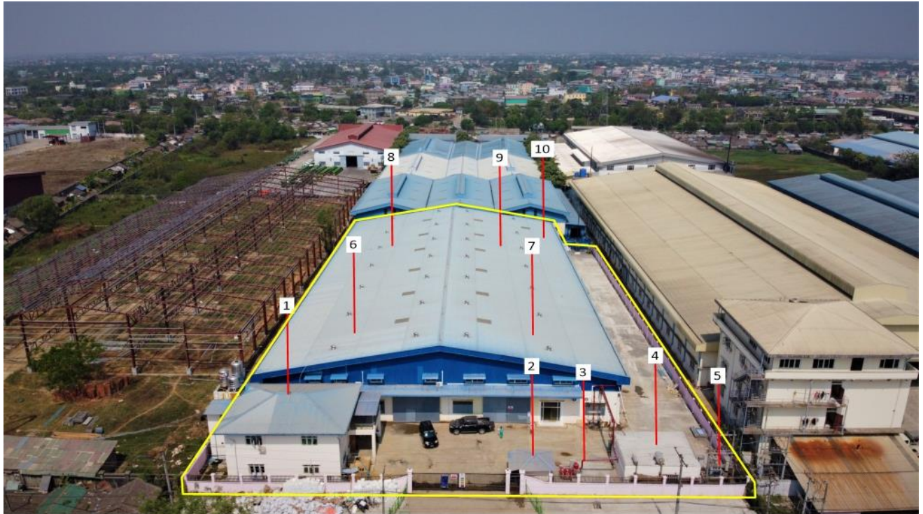
1.Office 2.Security Gate 3.Fire Safety Pump 4.Generator Room 5.Transformer 6.Warehouse 7.Packing Area 8.Sewing & Cutting Area 9.QC Area 10.Toilets
