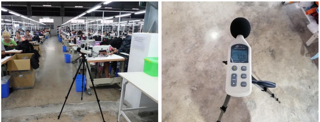
Figure 4-6 Sound level measurement photo
