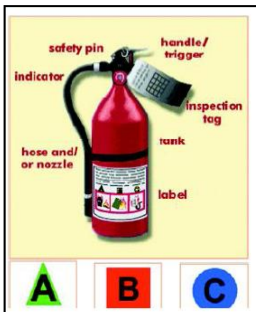
Figure 7-1 Components of a Fire Extinguisher
