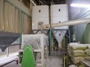
Figure 1-10 Dust collector system
