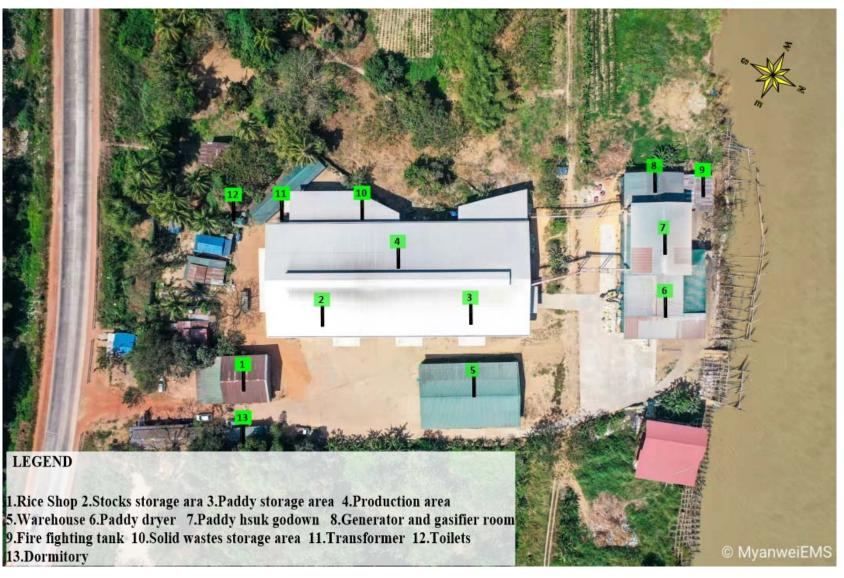
Figure 1-2 Production Layout Drawing of AGR Co., Ltd.
