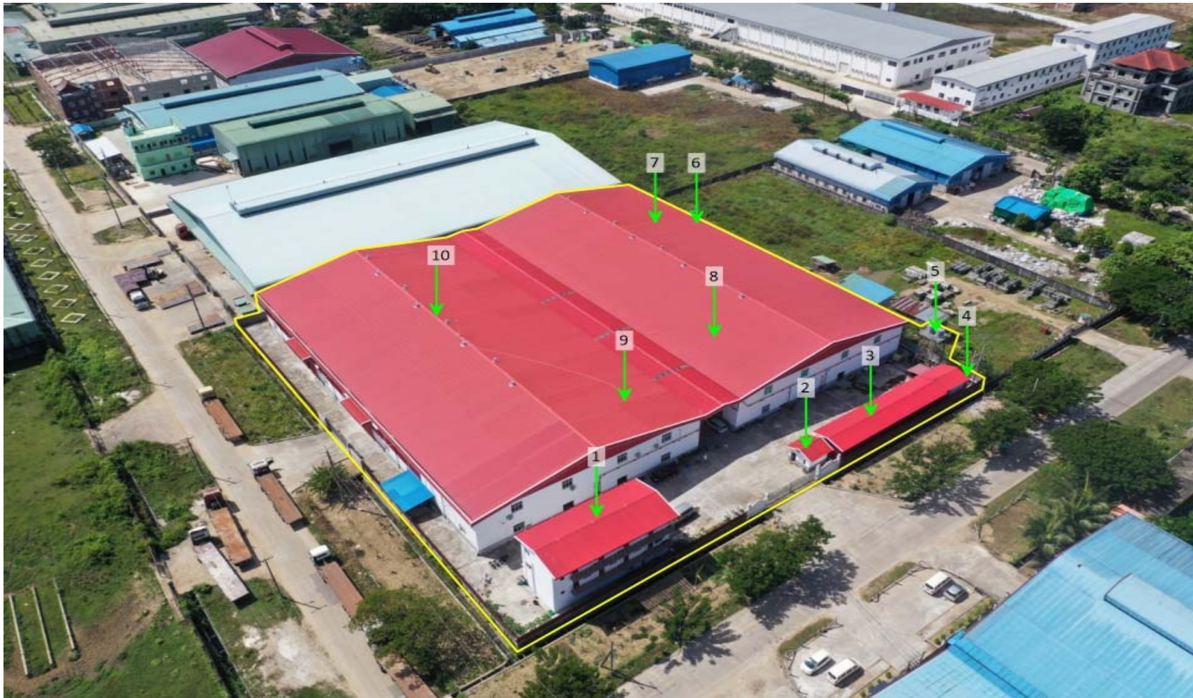
1.Dormitory 2.Security Gate 3.Generator Room 4.Transformer 5.Overhead Tank and Tube Well 6.Water Tank(Cooling System) 7.Raw Materials Storage Area 8.Toilets 9.Office 10.Production Area
