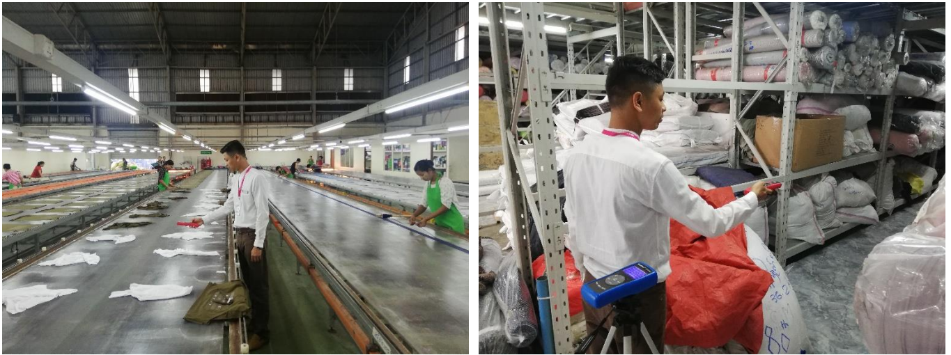
Figure 4-8 Light quality measurement
