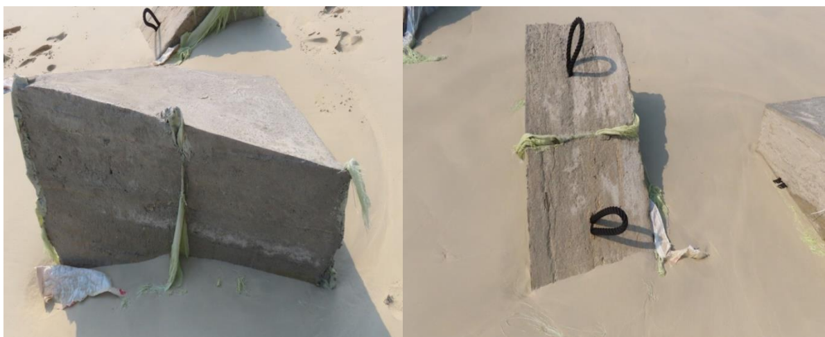
Figure 3-14: Sample Photo of Concrete Block using for Longline Laying (1m x 0.75m x 0.75m)
