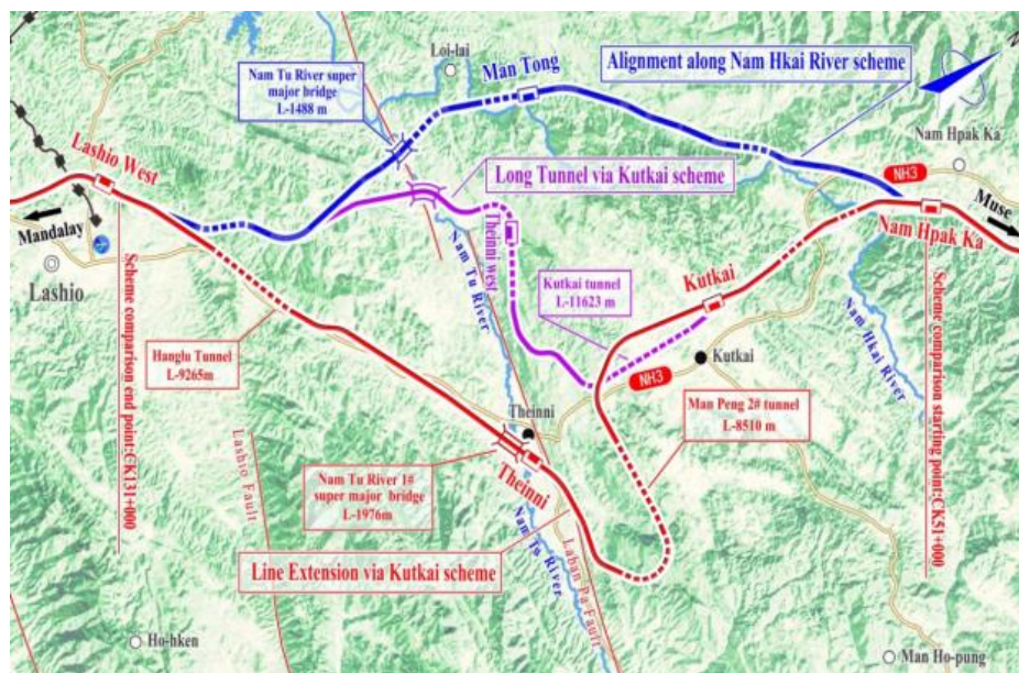
Figure 4.30 - Schematic Map for Alignment Scheme of Nam Hpak Ka-Lashio West Section
