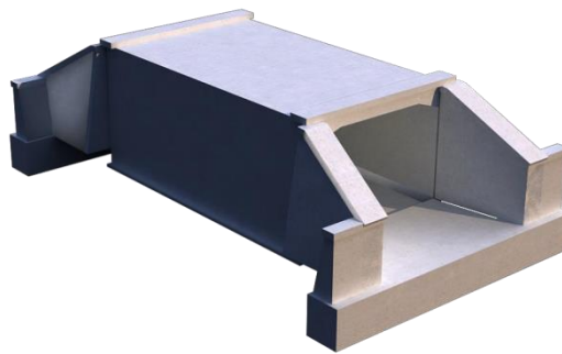
Figure 4.24 -Schematic Diagram of Railway Frame Culvert Structure
