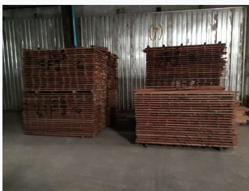
Figure – Air-drying by Sorting into Size
