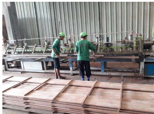
Figure – Joining with Finger Joint
