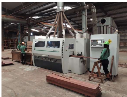
Figure – Planing with Four-side Planer Machine
