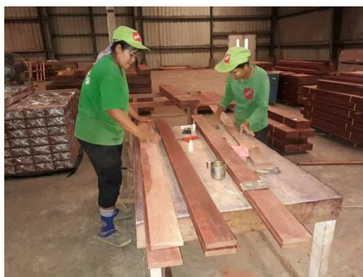
Figure – Polishing the Lumbers
