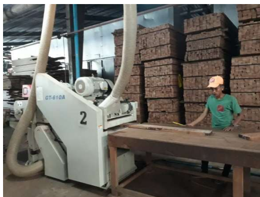
Figure – Adjusting Surfaces with Two-side Planer Machine
