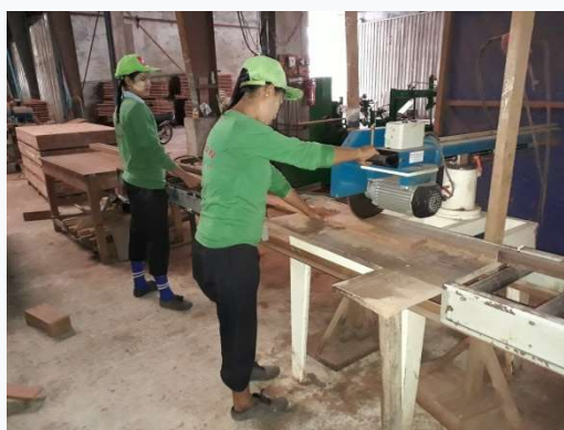
Figure – Cutting the Lumbers with a Sawmill
