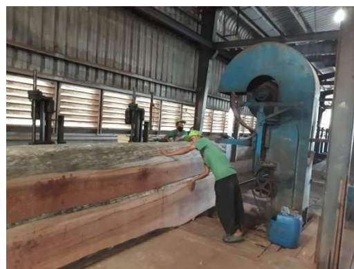
Figure – Breaking Logs with Sawmill
