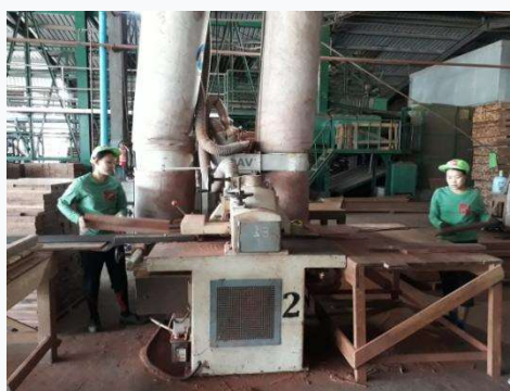
Figure – Edging Angles with One-way Lathe Machine
