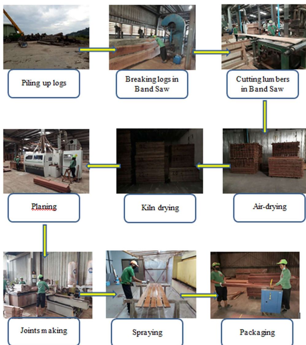
Figure 4.7. Photo Diagram of Value Added Wood Processes
