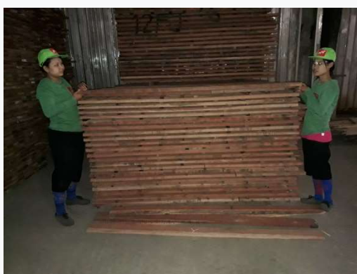
Figure – Arranging Lumbers for Air-drying
