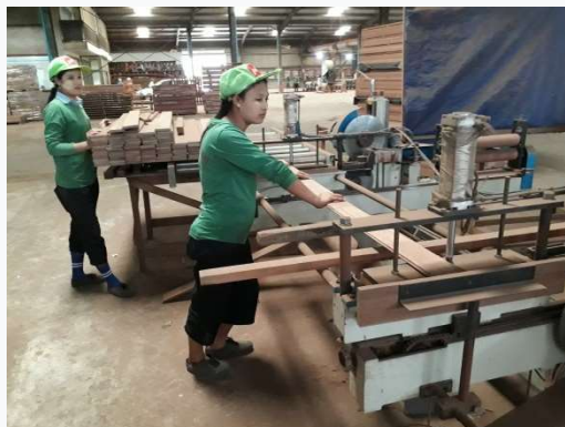
Figure – Edging the Angles with Wood Edger Machine
