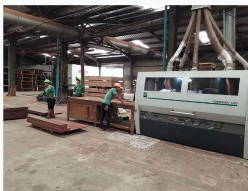
Figure – Planing with Four-sided Planer Machine
