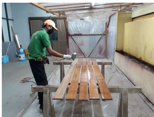
Figure – Spraying the Lumbers
