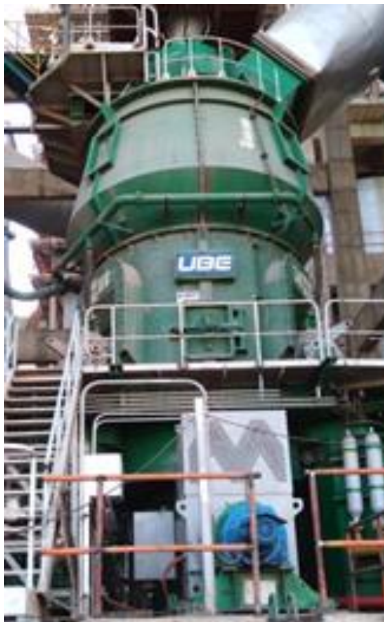
Figure 3.8-2: Coal Mill Used in MCL's Cement Plant
