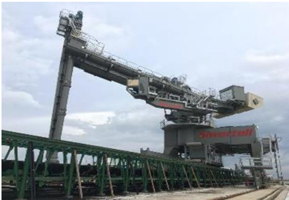
Figure 26: Screw Unload used in MCL's Cement Plant
