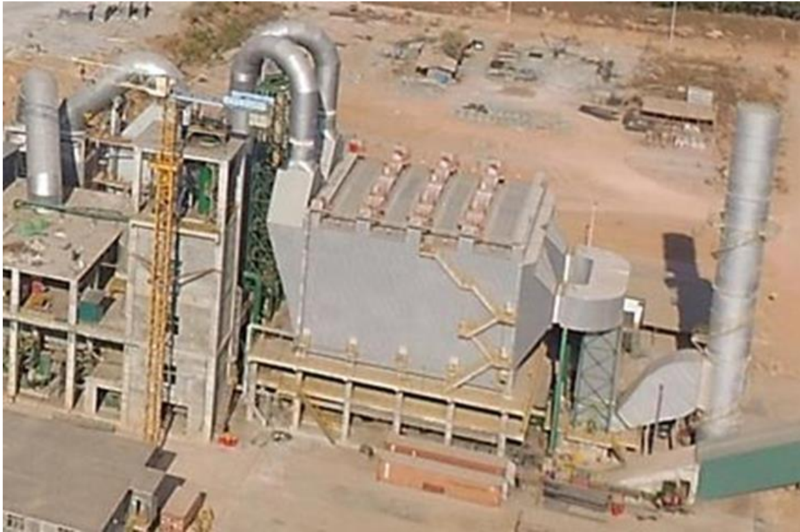
Figure 24: EP Clinker Cooler used in MCL's Cement Plant
