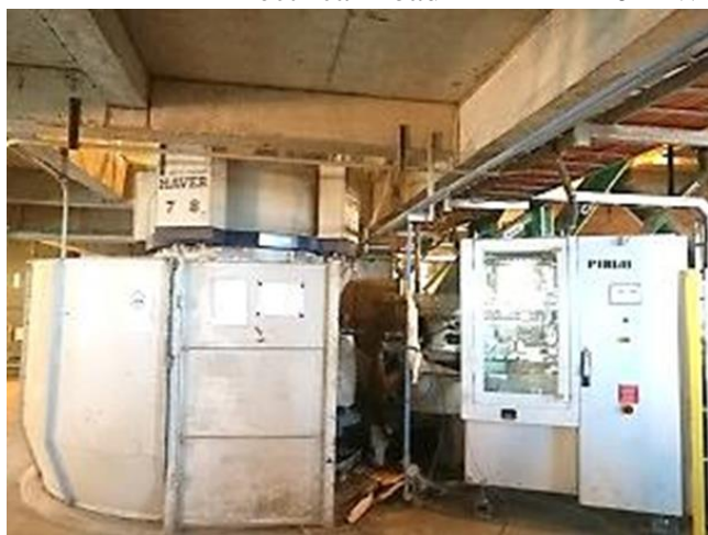
Figure 3.8-5: Rotary Packer and Cement Silo used in MCL's Cement Plant
