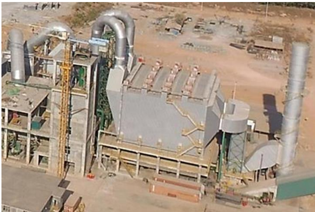
Figure 3.8-7: EP Clinker Cooler Used in MCL's Cement Plant
