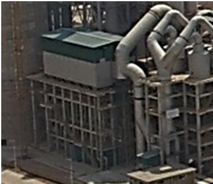
Figure 23: Bag Filter used in MCL's Cement Plant
