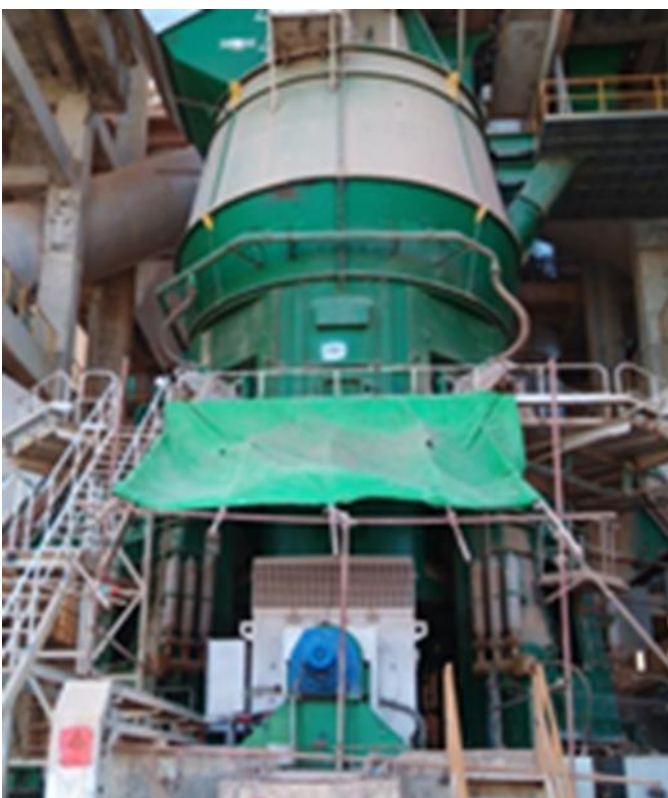
Figure 3.8-1: Vertical Raw Mill and Raw Material Hopper in MCL's Cement Plant
