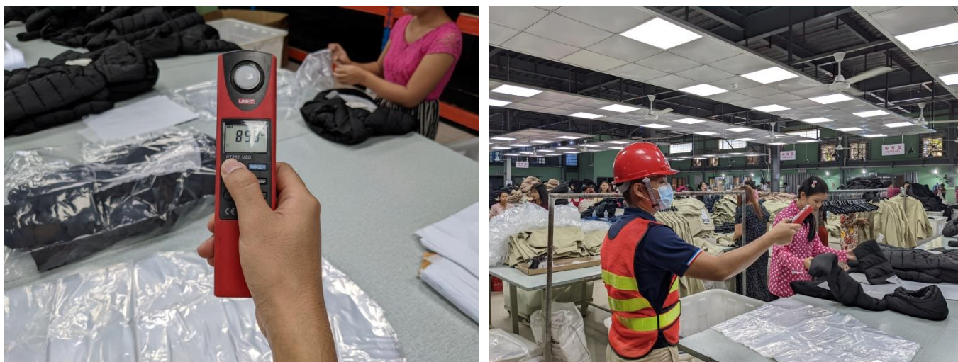
Figure 4-14 Light quality measurement
