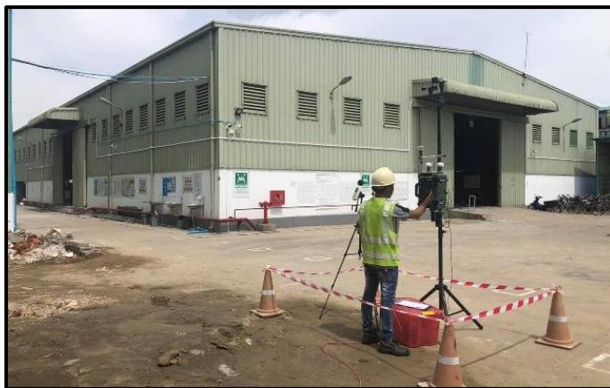
Figure 4-6 Ambient Air Quality and Ambient Noise Level Measurement
