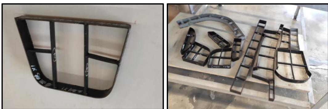
Figure 3-8 Molds for Pattern Making
