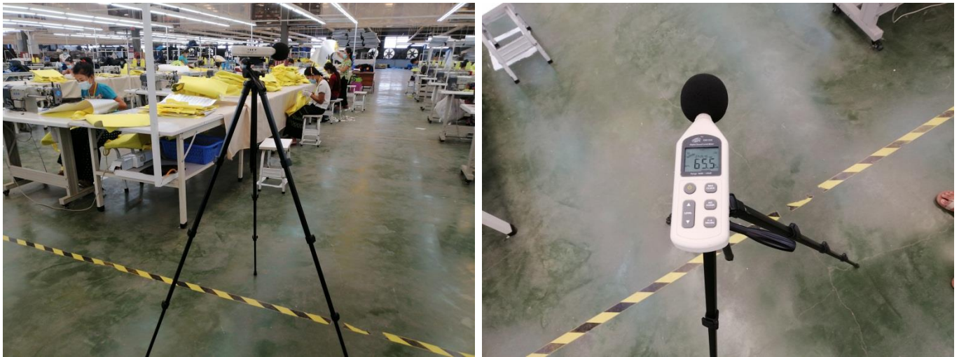
Figure 4-13 Sound level measurement photo
