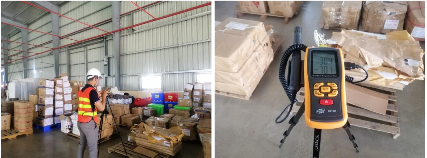
Figure 4-9 Temperature and Humidity Measurement in Operation Area
