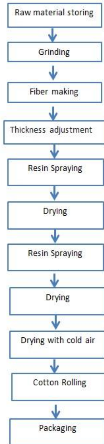
Figure 4. Process Flow Diagram for Yu Chang (Myanmar) Spray Cotton Co. Ltd The production process produces non liquid effluent and slightly gaseous emission from boiler and generator. Discharged waste water of factory was disposed to municipal drainage.
