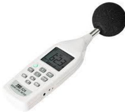
Figure 12. Noise Level Meter for Measuring Noise
