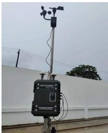
Figure 10. Air Monitoring with Haz- Scanner in Factory Compound
