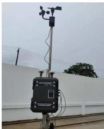
Figure 8. Air Monitoring with Haz- Scanner in Factory Compound
