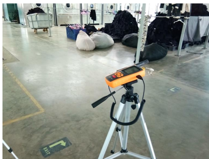
Temp and HD measure at Cutting
