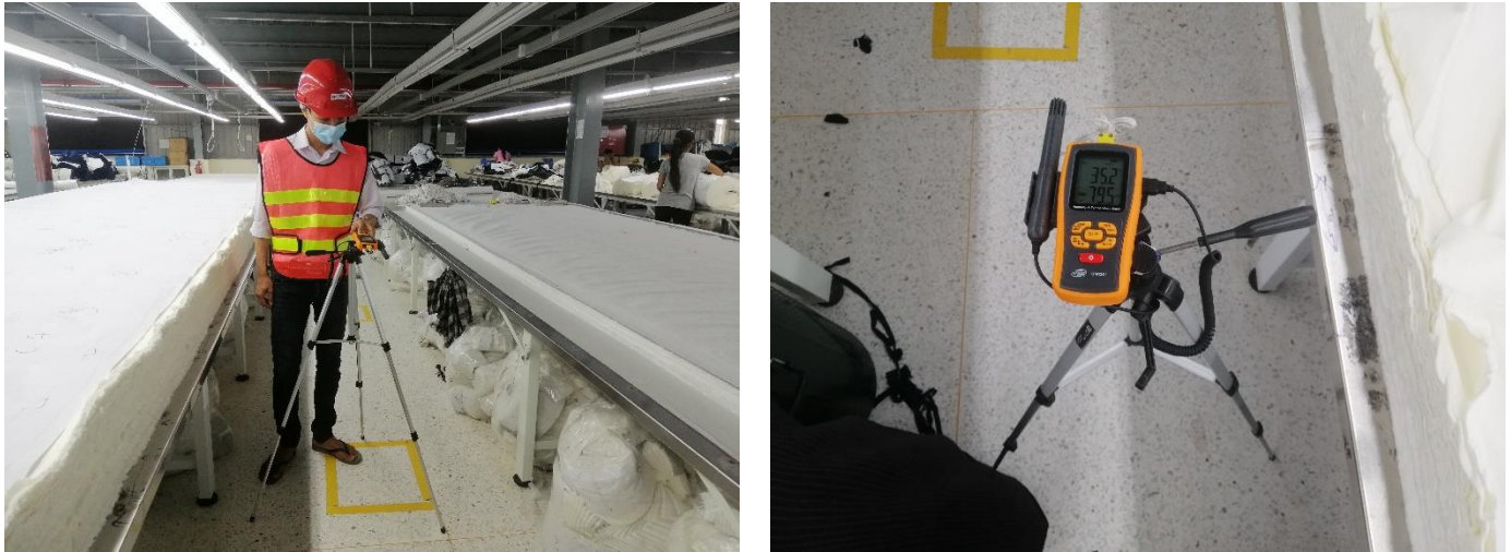
Figure 4-1 Temperature and Humidity Measurement in Operation Area
