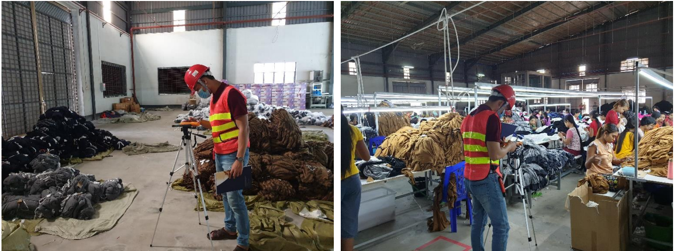
Figure 4-1 Temperature and Humidity Measurement in Operation Area
