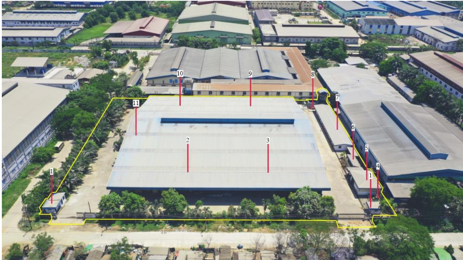
1. Security Gate 2. Cutting & Ironing Area 3. Packing Area 4. Transformer 5. Generator Room 6. Toilets 7. Dormitory 8. Fire Safety Pump & Water Tank 9. Sewing & QC Area 10. Warehouse 11. Office
