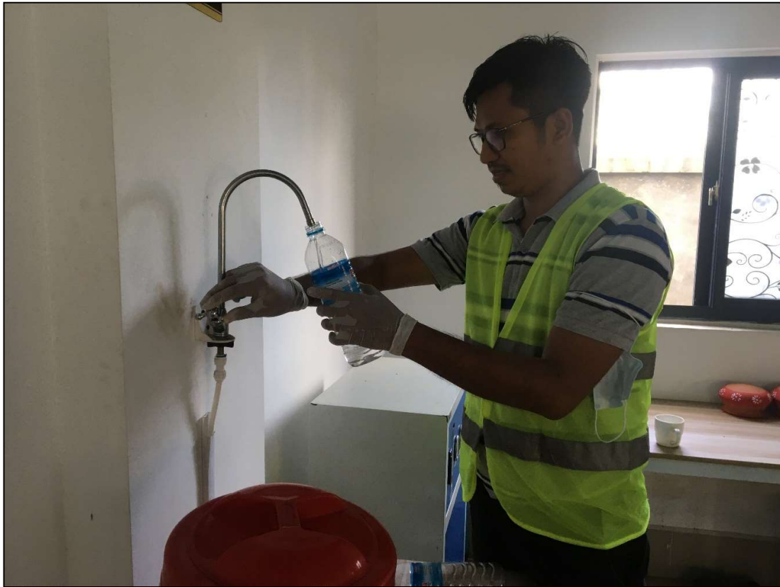
Figure 1-8 Water Sample Collected from Drinking Water Pipe
