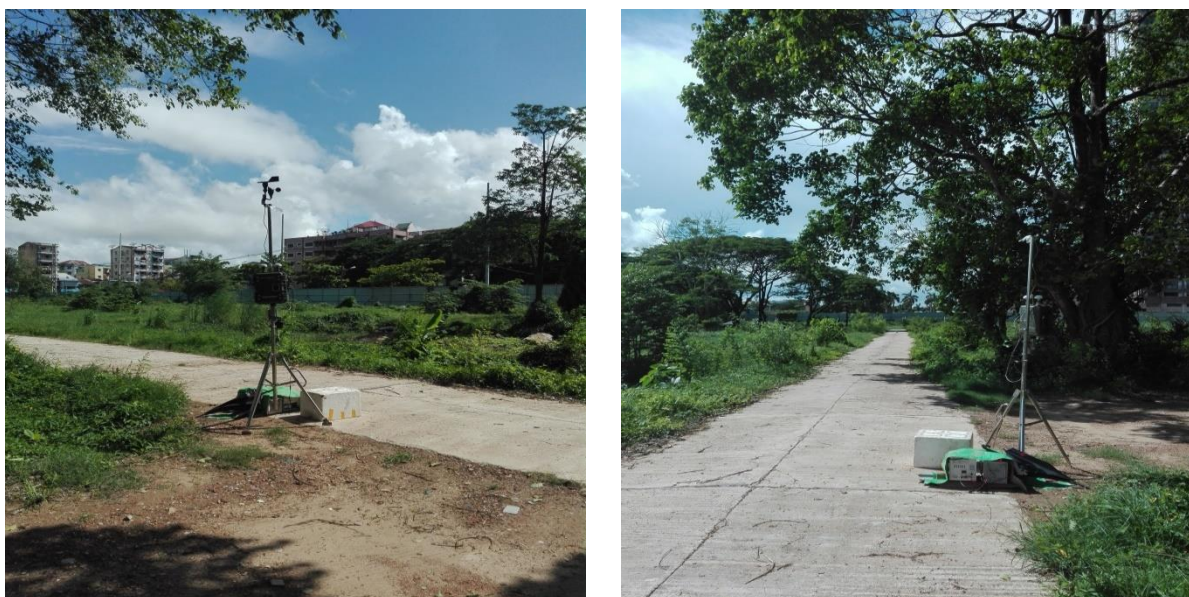
Figure 3: Air Quality Monitoring inside the site boundary
