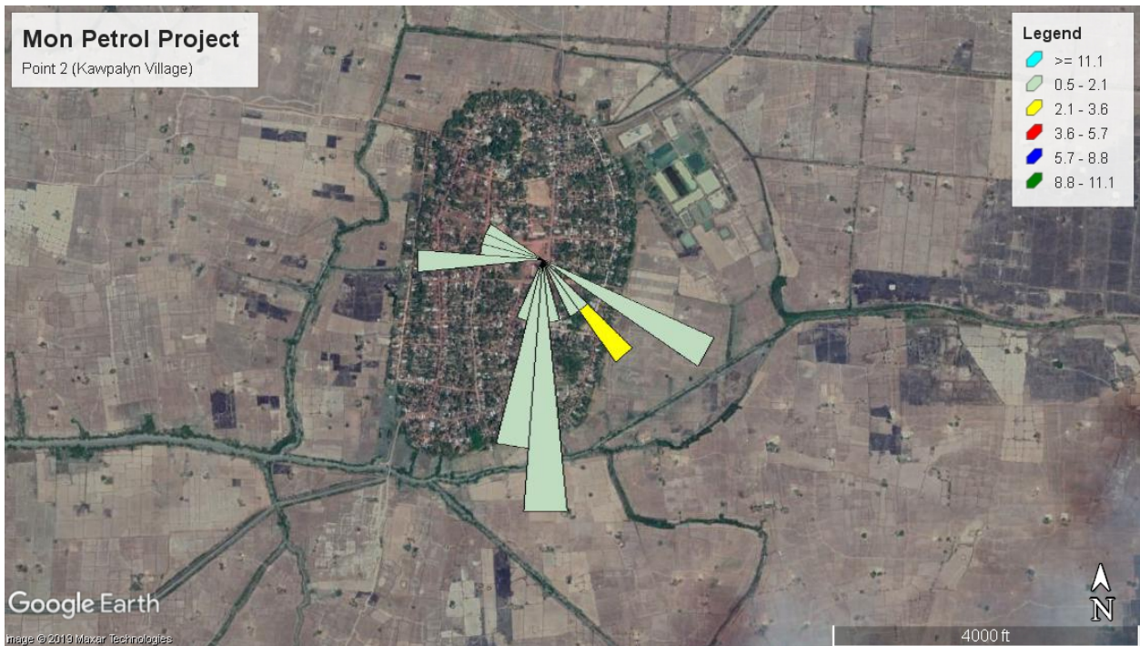
Figure 6. 13 Wind Speed and Wind Direction (Blowing From) at Kawpalyn Village
